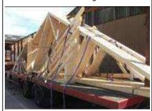
3. The Manufacturer will supply truss packs secured to the trailer with 3 core rope or appropriate banding. You shall familiarise yourself with which rope / banding attaches which pack to the centre bars.
