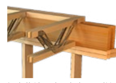
TF5 - Top Chord Support on Standard Panel with Rim Boards - External Wall
