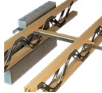
SD15 - Restraint Strap with Additional Noggins
