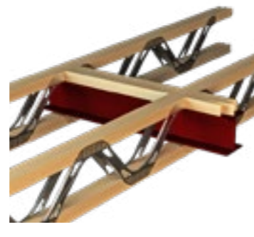
SD13 - Top Chord Support onto Steel
