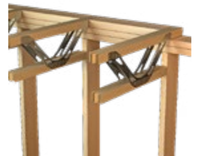
TF3 - Top Chord Support on Over-height Panel - External Wall
