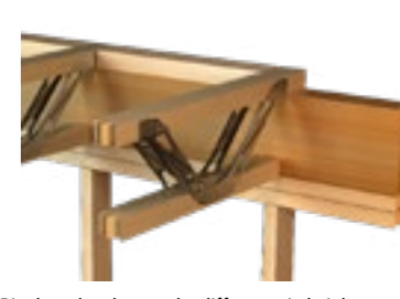
TF6 - Top Chord Support on Standard Panel with Rim Boards - Party Wall
